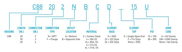
Note: If DOE, it is only required once in the part number and will specify both top and base. Cartridges are not included but must be specified as to the type using when ordering the housing. Carbon steel not recommended for water use as the epoxy coating is not designed as a corrosion inhibitor.
