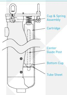
\*\*Note: Type of element top which will be used must be noted at the time of the housing order.
